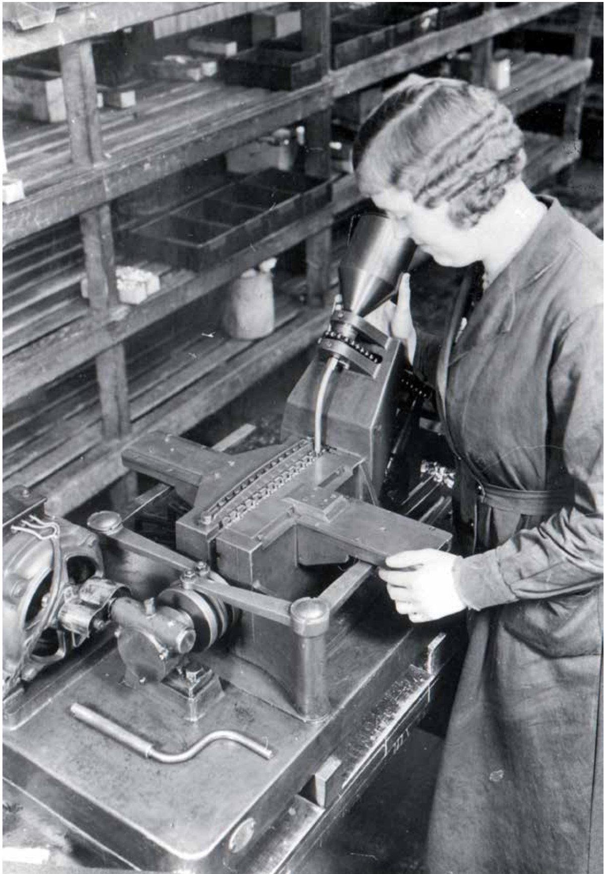
Boring cylinders at the Redditch Factory, 1937
